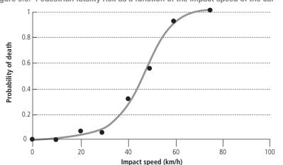
Figure 9.6. Pedestrian fatality risk as a function of the impact speed of the car<sup>22</sup>
